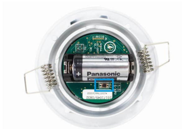
The sensor and the energy saver will then try to synchronise. Synchronisation is correct when the red sensor flashes very quickly for about five seconds. The red pilot light must go off then. Repeat the same procedure with all the sensors in the same room that must be synchronised with the same energy saver. Remove the card from the energy saver once all sensors have been synchronised.
